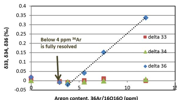
Figure 3. Dual inlet measurement:  $\delta 33$ ,  $\delta 34$  and  $\delta 36$  of O<sub>2</sub> reference gas spiked with argon with respect to pure oxygen reference gas, plotted against  $^{36}\text{Ar}$  content of the spiked oxygen gas.
