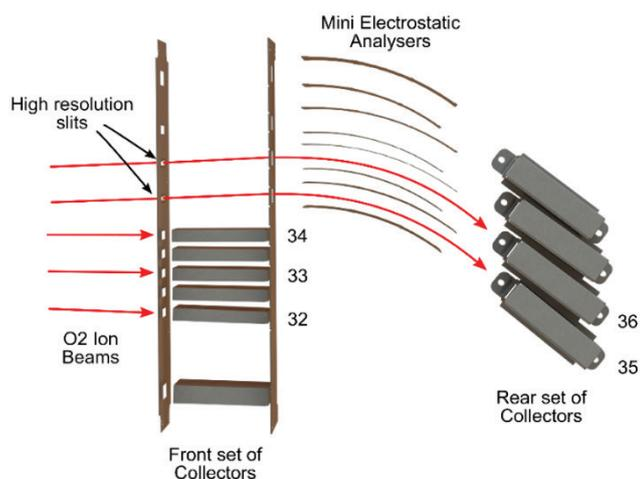
Figure 1. Schematic view of the Perspective IS collector array showing the O<sub>2</sub> masses 32 to 36. Low abundance "clumped" signals mass 35 and 36 enter the collector array through high resolution slits and are filtered through "mini-ESA"s.
