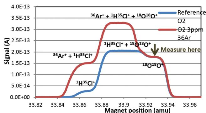
Figure 2. Mass 36 ion signal at MRP  $\approx 3600$ ; comparison between pure oxygen reference gas (blue) and oxygen containing 3 ppm  $^{36}\text{Ar}/^{16}\text{O}^{16}\text{O}$  (red). IRMS measurement takes place on the right shoulder ( $^{18}\text{O}^{18}\text{O}$  only). Mass 32  $^{16}\text{O}^{16}\text{O}$  ion current  $\approx 4 \times 10^{-8}$  A (8 V).
