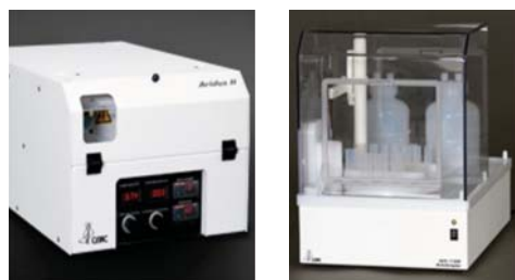
Figure 2: Sample introduction system used for the dry plasma experiment (Cetac Aridus II, left) and autosampler used for all measurements (Cetac ASX112, right).
