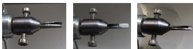
Fig. 1: A high purity tantalum sample holder (left) acts as an electrode in the analysis of alumina powder (center) and sapphire wafer (right).
