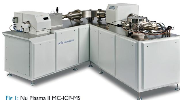
Fig 1: Nu Plasma II MC-ICP-MS
