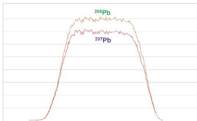
Fig 3: Typical Pb peak shapes achieved using the Plasma 3 multiple-Daly system.
