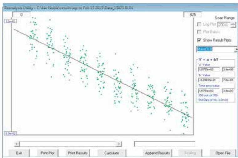
The standard Nu Instruments Calculation Editor (NICE) software provides user-definable data reduction functions. Both raw and calculated data are available for each sample run along with full logging of instrument settings. data can be analysed on or off-line and can be easily exported for further analysis to third party software packages.
