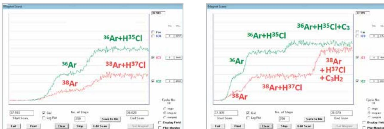
Mass scans showing resolution of  $^{36}\text{Ar}$  and  $^{38}\text{Ar}$  from interferences
